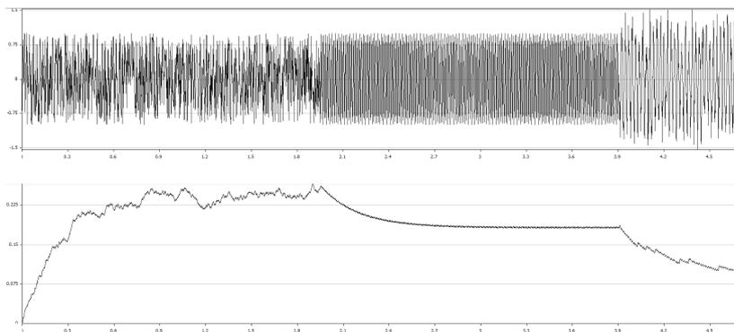
**Fig. 2.** This figure shows the momentary frequency estimation for a signal containing two transients, from white noise to a pure sinusoidal wave and then to a sine wave with a different frequency superimposed with white noise.
