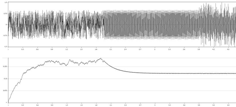
**Fig. 3.** This figure shows the momentary frequency estimation for a signal containing two transients again. This time the third part is a superposition of the white noise from part 1 and the sine from part two. As a result the white noise is filtered entirely.
