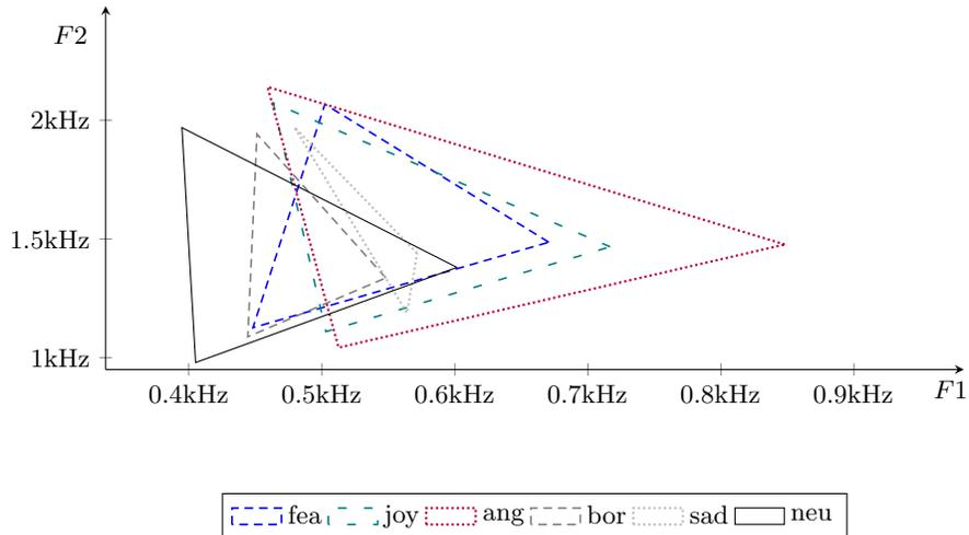
**Fig. 1.** Classical vowel triangle forms for male speaker's and various emotional states. The triangles are built on the mean positions of *i*, *a* and *o* vowels in the F1/F2 space. Estimated on speech material from the EMO-DB database
