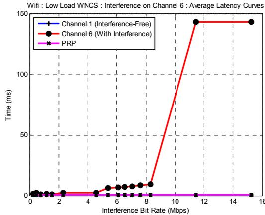
Fig. 7. Wi-Fi Low-Load – single interference
