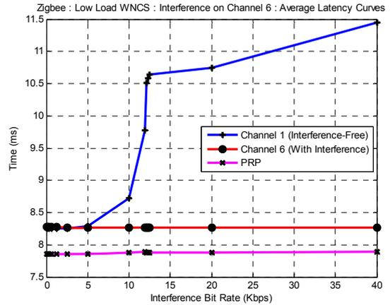
Fig. 8. ZigBee Low-Load – single interference
