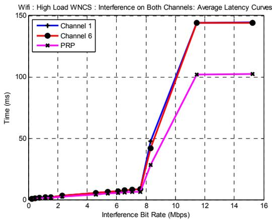
Fig. 4. Wi-Fi High-Load – dual channel interference
