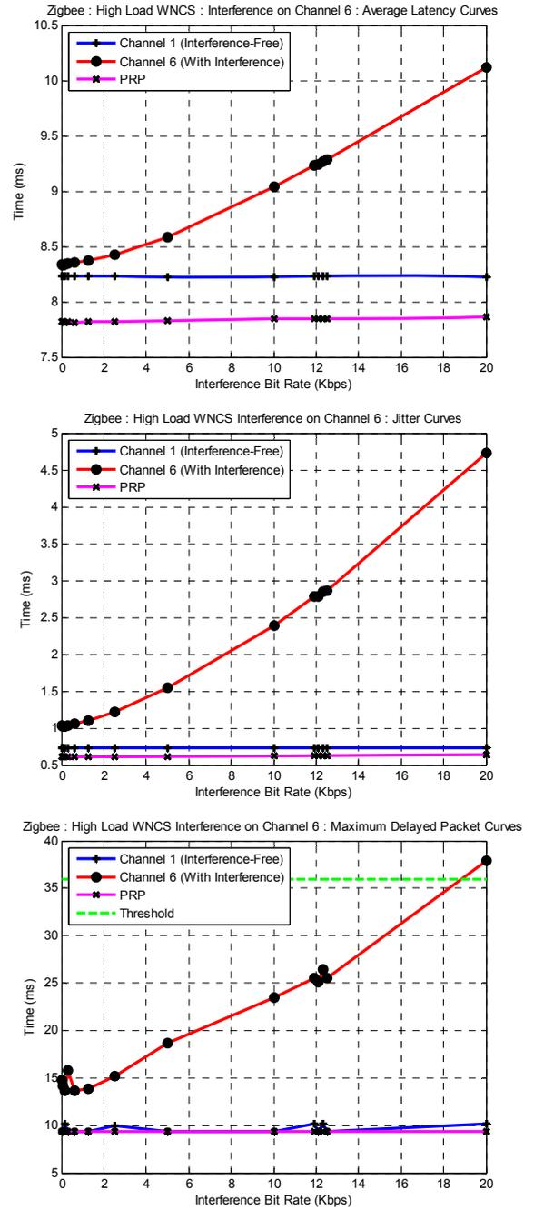
Fig. 5. ZigBee High-Load – single channel interference
