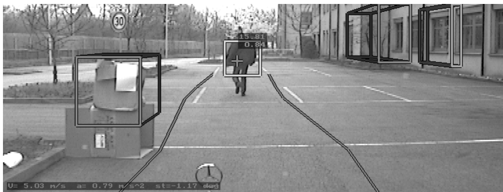
Figure 7.15: Avoidance scene with a human as a leader vehicle passing close to a cardboard box on the left. Due to the larger width, the ego-vehicle performs a swerve maneuver to avoid the box. The elastic band path is depicted projected to the ground. The leader vehicle and the ego-vehicle are about 12m apart.
