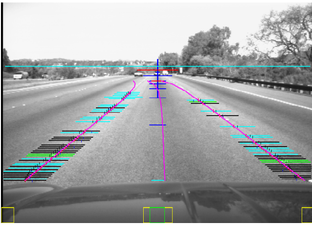
Fig. 7. California freeway scene on Interstate I 280. Bots dot algorithm active. The offset estimate is accurate.
