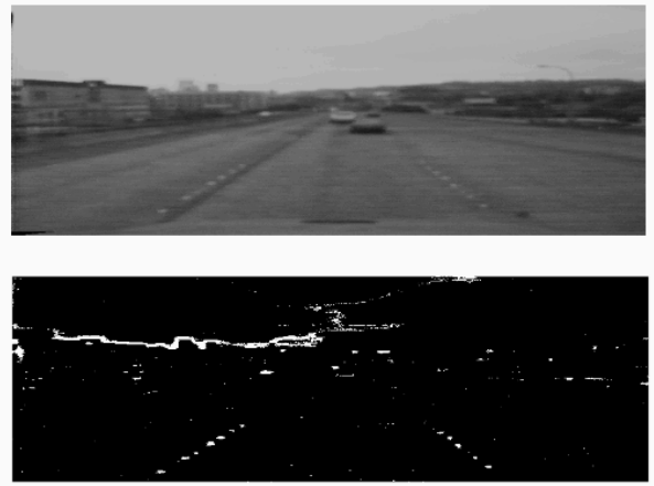
Fig. 3. Filter result of the bots dot detection run over the whole image. For our algorithm, we only search within our lane marking windows
