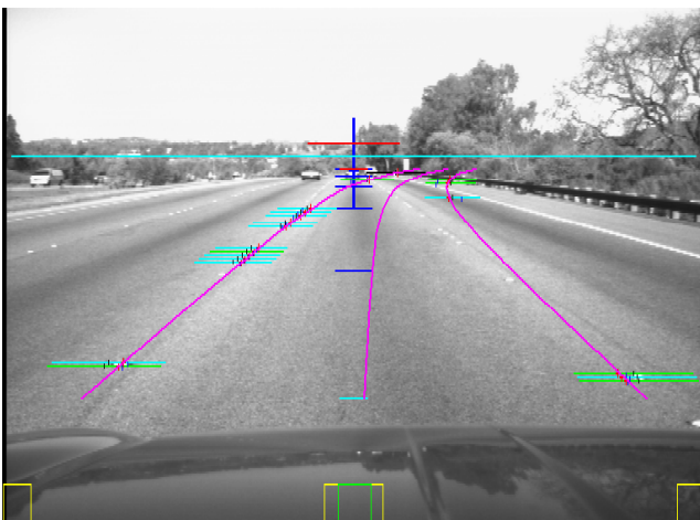
Fig. 8. California freeway scene on Interstate I 280. Standard lane recognition only. Hardly any measurements are found with the edge-based feature extraction
