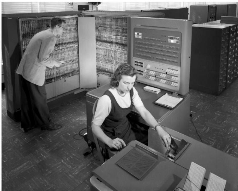
„The type 704 Electronic Data-Processing Machine is a large-scale, high-speed electronic calculator controlled by an internally stored program of the single address type.“
